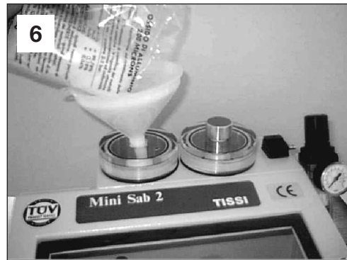
6 Fill containers with appropriate grain size of sand
