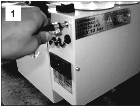
1 Connect air pressure hose (max 10 bars)
