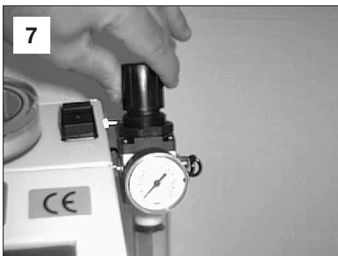
7 Regulate air pressure (min 2 – max 6 bars)
