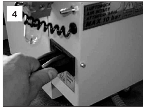
4 Insert plug respecting voltage on back plate
