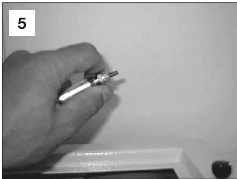
5 Mount appropriate nozzles on ejector pen
