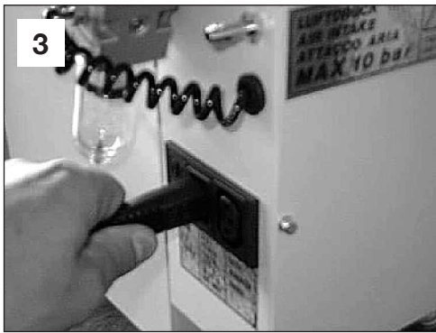
3 Connect aspirator plug in the sandblaster socket
